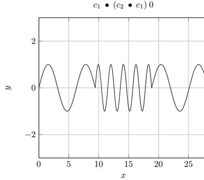
This type of signal is commonly seen in *frequency modulation*: the varying frequency is used to encode information for electromagnetic transmission. Note that  $c_1$  gives control for some time to  $c_2$ , and then ‘takes it back’.
