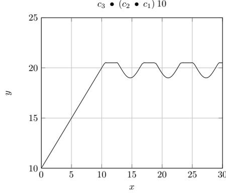
Clearly,  $c_3$  can be regarded as a supervisor system that, for the sake of efficiency, only acts when temperatures exceed the threshold, using just enough power to keep the temperate below the limit. Actually, note that  $c_3$  is able to play a supervisory role precisely because it is non pre-dynamical. Of course in this specific case, we assume that  $c_3$  has an idealised behaviour, which, despite pedagogical, is quite unrealistic.
