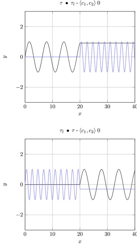
Clearly,  $\tau \bullet \tau_l \neq \tau_l \bullet \tau$ ; but note that the plots illustrate an interesting aspect: specification  $\tau \bullet \tau_l \cdot \langle c_1, c_2 \rangle$  reads ‘first let the component in the left to act, then the one in the right’; and conversely for  $\tau_l \bullet \tau \cdot \langle c_1, c_2 \rangle$ . Moreover, note that each component ‘waits’ for the other by stalling the corresponding evolution. This introduces yet another synchronisation mechanism.
