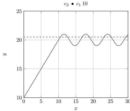
If, however, temperatures over  $20.5^\circ\text{C}$  occur, composition  $c_3 \bullet (c_2 \bullet c_1)$  puts the system back into the right track as illustrated in the following plot.
