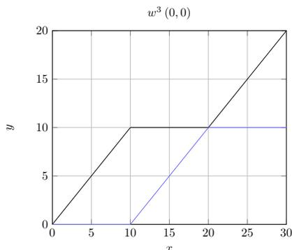
On a different note, it is natural to consider that the pump takes some time to switch from one tank to the other: for illustration purposes let us assume that time to be ten seconds. To simulate such a delay we can define a variant of  $copy$ , denoted by  $copy_{10}$ , that always outputs evolutions with duration ten. Then, again for input  $(0, 0)$ , system  $(copy_{10} \bullet w)^3$  outputs
