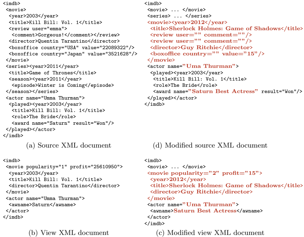
Fig. 3: Example of a bidirectional transformation between XML documents.
